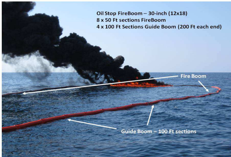
Figure 8. Source: Oil Stop L.L. C. Showing Controlled Burning inside its Fire Boom
